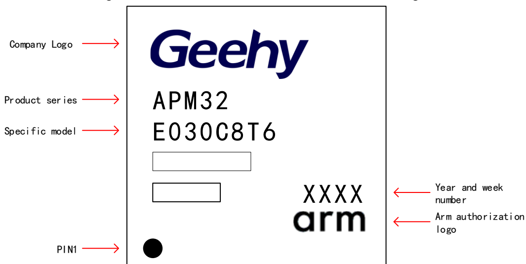
Figure 25 LQFP48 -48 Pins, 7 x7mm Schematic Diagram
