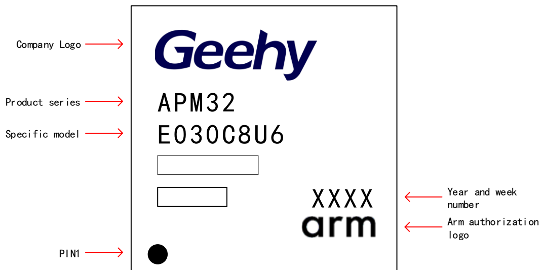
Figure 28 QEN48 - 48 Pins, 7 x 7mm Package Schematic Diagram
