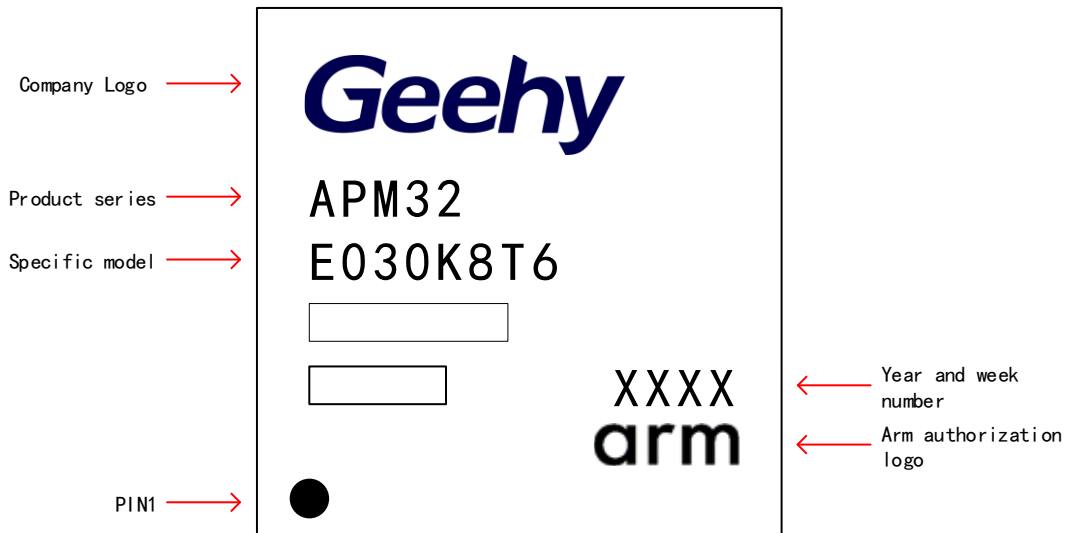
Figure 31 LQFP32 - 32 Pins, 9 x 9mm Package Schematic Diagram
