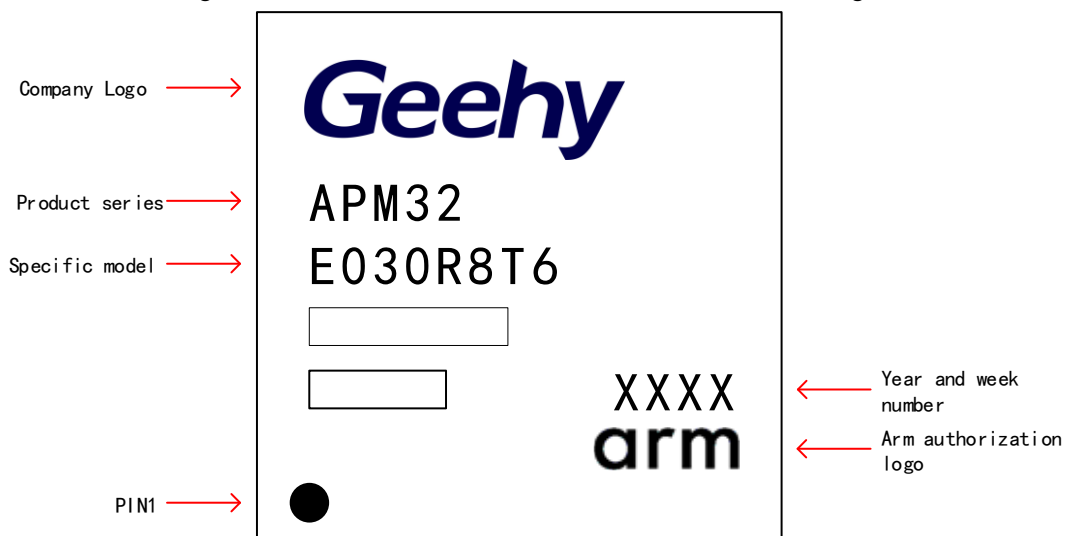
Figure 22 LQFP64 -64 Pins, 10 x10mm Schematic Diagram
