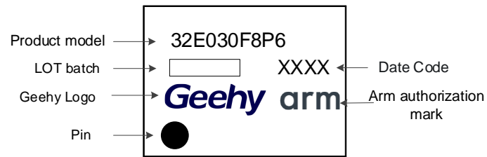
Figure 40 TSSOP20 – 20 Pins,4.4 x 6.5mm Package Schematic Diagram
