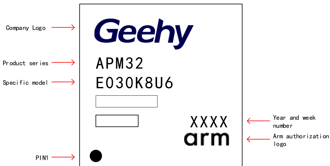
Figure 34 QFN32 - 32 Pins, 5 x 5mm Package Schematic Diagram
